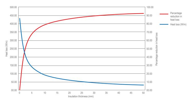
This would suggest that it is more important to ensure maximum coverage of pipework with insulation than it is to insulate easy-to-reach portions of piping with very thick insulation, leaving some pipework bare.
