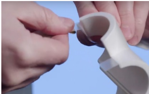
5.1 Apply tape cut down to 12.7mm width to the tee fitting.
